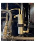
We installed a special system below the cab on the fireman's side that allows the boiler water to be sampled while it is at operating pressure/and temperature.
