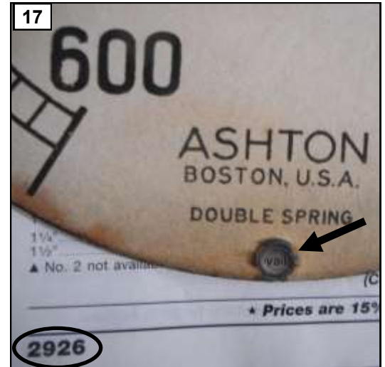
Above: The first picture (16) shows one of the old gauge faceplates on an open copy of the McMaster's catalog. The arrows point to the screw holes for which ferrules are needed. The second (17), shows a close-up with the page number in the lower left corner.
