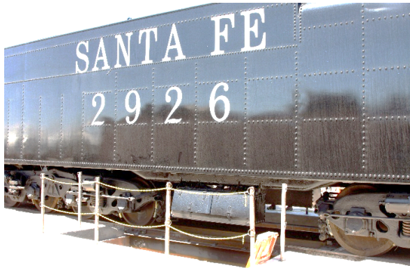
Exterior of the tender showing baffle rivet pattern
