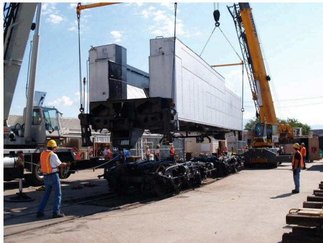
The water canister being removed during the tender overhaul
