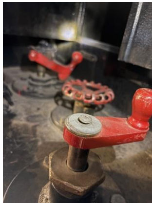
Injector inlet valve, tell-tale petcock inlet valve, bootwasher valve and
