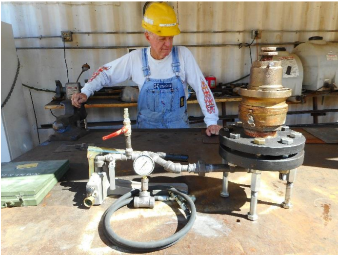
...that was used to set valve release pressure with a pressure transducer and nitrogen pressure.
