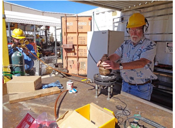
...that was used to set valve release pressure with a pressure transducer and nitrogen pressure.
