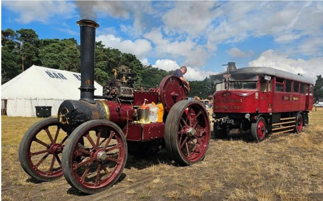
Figure 5. Vertical steam boiler city bus (background) pushing a traction engine into the water refill area
