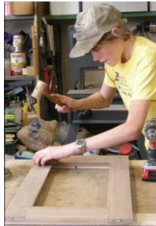
Replication of Santa Fe 2926 Window Frames: These photos show Sam Baczkiewicz hard at work in his shop measuring, drilling, joining, and sanding Santa Fe 2926 window frames.
