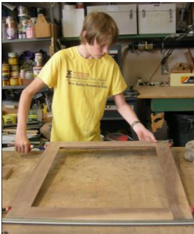
Replication of Santa Fe 2926 Window Frames: These photos show Sam Baczkiewicz hard at work in his shop measuring, drilling, joining, and sanding Santa Fe 2926 window frames.
