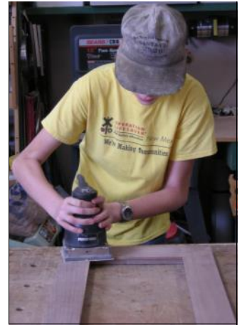
Replication of Santa Fe 2926 Window Frames: These photos show Sam Baczkiewicz hard at work in his shop measuring, drilling, joining, and sanding Santa Fe 2926 window frames.
