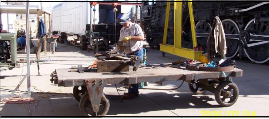
In this picture, Jim Hills, a SNL Contractor works on the brakes from the tender. His workbench is a very heavy steel trailer that was used to shuttle parts around the AT&SF backshops. Jim also restored the metal portions of the 2926 cab.
