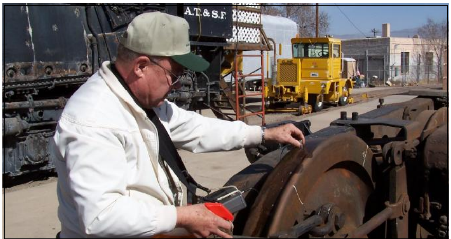
Surplus equipment was acquired from SNL to perform ultrasound testing on parts of 2926. With the equipment came volunteer ultrasound specialist John Gieske. Here, he is checking the wheels of the 2926 water and fuel tender. The yellow car mover in the background was donated to WHEELS Museum by SNL, and leased by NMSLRHS. NMSLRHS member Dick Sons operated the car mover at SNL.
