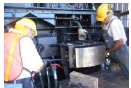
Above: More radial buffer work at the front of the tender.
