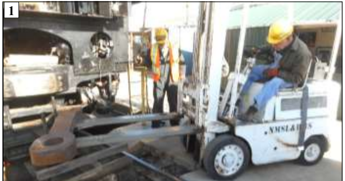
1 Drawbars are delivered to the rear of 2926 by forklift.
