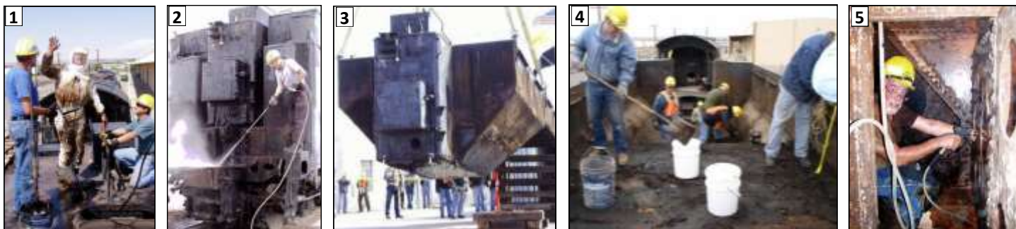
Bunker Cleaning And Preparation, Stage 1, 2003: The cleaning began in early 2003 by removing caked oil inside and out, (1 & 2). The fuel bunker was then lifted, (3) from the tender and placed on cribbing for more cleaning, Surprise!! More caked oil and assorted trash in the fuel bunker pocket, (4). Inside the water bunker, the crew scraped, scrubbed, and needle scaled hundred of pounds of scale, rust, and trash.
