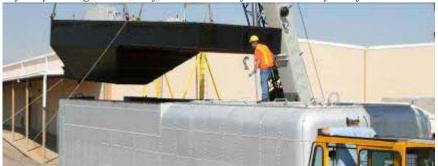
*NMSL&RHS member Clem Harris watches closely as the crane operator slowly lowers the fuel bunker into its place in the front of the tender.*
