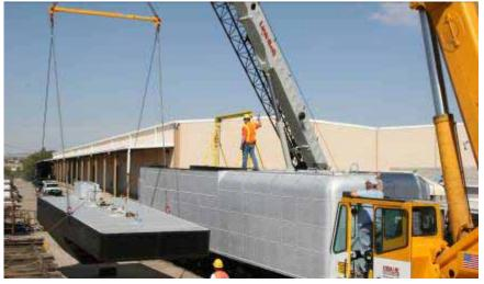
Lifted by the larger crane, the fuel bunker heads for its nest at the front of the tender.
