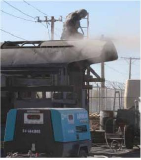
the care of 2926 in years to come. Above: Recently, R&R was back again. This time they puickly blasted the cab of 2926 free of many years of paint and corrosion.
