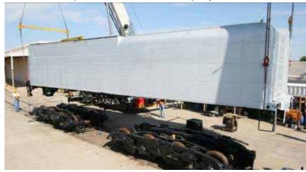
THIS IS ONE BIG WATER TANK! The two crane operators coordinate the lift smoothly via radio to move the tender body over its trucks.
