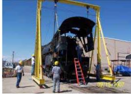
Once cab is lifted clear, 2926 is pulled forward. The cab was set on cribbing out of picture at left.
