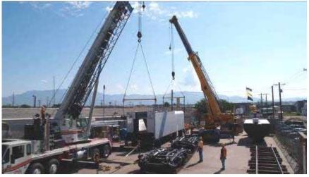
Against a Sandia Mountain backdrop, the two cranes operate in unison to lift the huge tender body. It floats slowly from the cribbing where it was restored to its freshly restored trucks already back on tracks at bottom center of the photo.
