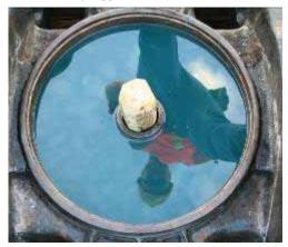
Lubing up: (L) Clem Harris pours oil into the bolster pocket on one set of trucks. (R) Pocket full of oil with Clem's reflection in fresh oil. The wooden pin in the center is used for alignment with the upper portion of the bolster on the bottom of the tender.
