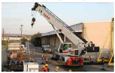
On site, ready to lift. The 75-ton crane is positioned for first lift, one set of the tender's two sets of eight-wheel Buckeye trucks. Trucks weigh approximately 19 tons each.
