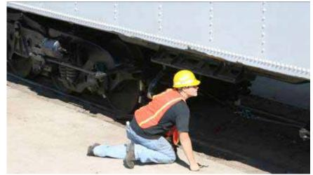
Travis Atwell kneels at the side of the rear truck to keep an eye on the alignment pin as the tender body slowly settles onto the trucks. Another crew member observed the other truck as the crane operators eased the body down an inch at a time.
