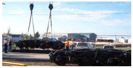
With both cranes lifting, the second set of trucks follows the first.
