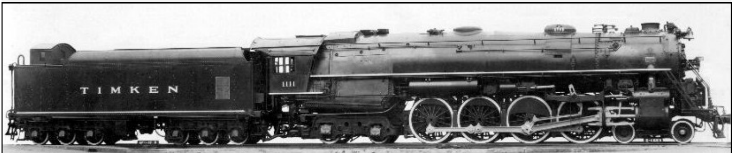
Timken Roller Bearing Company’s Famous Four Aces: Timken chose the 4-8-4 design so it could be used by a variety of railroad work, including heavy freight and fast passenger service, to demonstrate their roller bearings.
