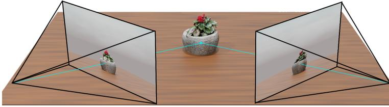
Photos of the real world can be quite complex. Photogrammetry applications use sophisticated algorithms to process images of an object in order to find common points in multiple photos and “stitch” these images together to create a 3D model. Look at the turquoise lines in the image to the left. The lines each target the same point from a different perspective.
