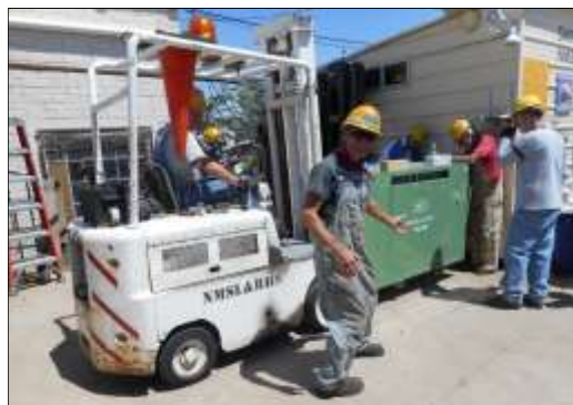
The small forklift is used to move the Sullair air compressor into place next to the WHQ.
