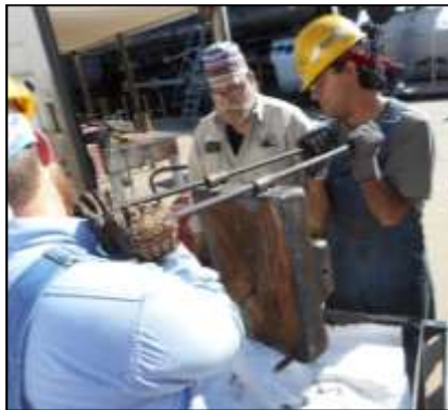
Above are the two dynamos that will provide electrical power when operating. At right is a photo of recently fabricated jacking. Some trimming and tailoring was necessary to fit the new jacking over the steam chest.
