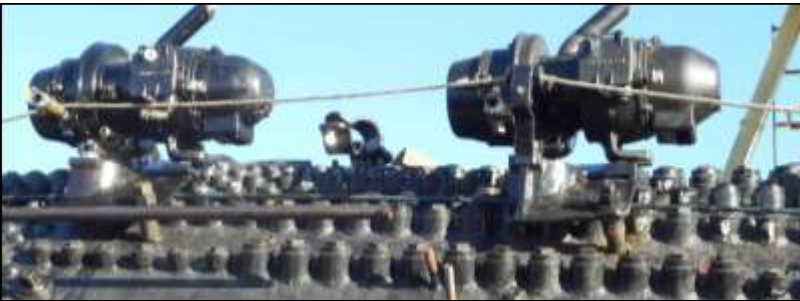
Above are the two dynamos that will provide electrical power when operating. At right is a photo of recently fabricated jacking. Some trimming and tailoring was necessary to fit the new jacking over the steam chest.
