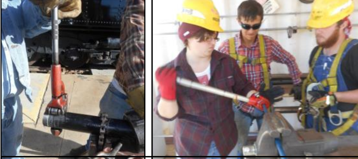
Above and Below: Just threading and connecting the pipes occupied many hours of volunteer time, Below Right: Nate finds pipefitting workspace underneath the cab a bit cramped.
