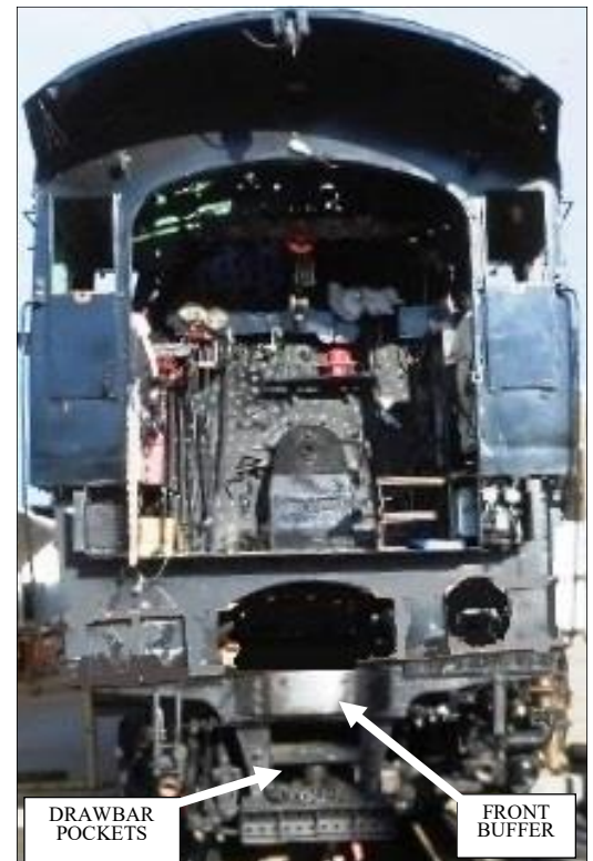
This view is different now. Cab controls, gauges, and appliances have been installed. .
