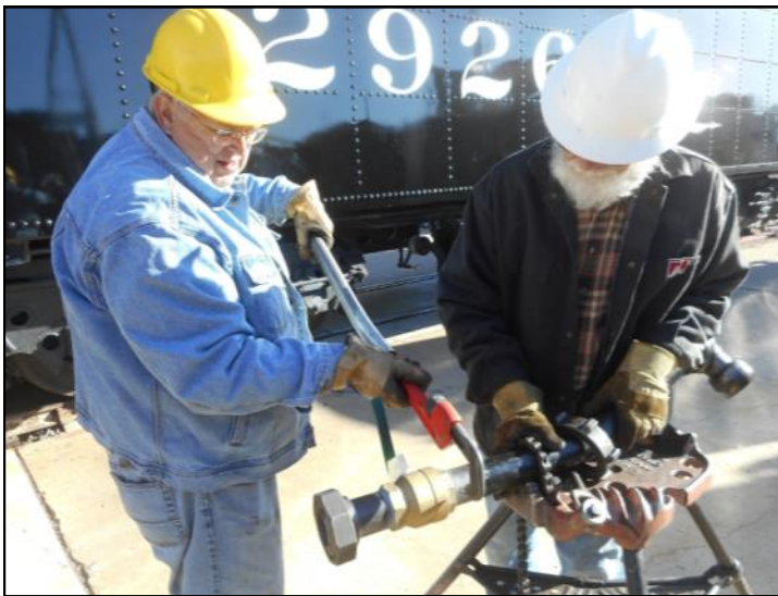
Above and Below: Just threading and connecting the pipes occupied many hours of volunteer time, Below Right: Nate finds pipefitting workspace underneath the cab a bit cramped.
