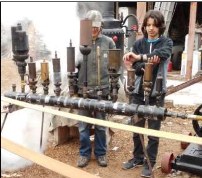
A Steamy Greeting For The New Year: Scotty Altenbach stands ready to start sounding a variety of steam whistles as Dan Toyama counts down to exactly noontime January 1, 2015. The whistles are mounted on a manifold connected to the boiler by a high pressure hose. Drive belt for saw is in foreground.
