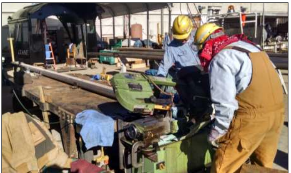
TOP: Flue tubes are removed from the storage container in background and racked for cleaning, inspection, and cutting to proper length.. BOTTOM: A metal wagon once used to haul parts about the Albuquerque Back Shops, is pressed into service as a work table where tubes can be securely clamped for accurate measurement and cutting with a metal saw. The fresh cut ends are cleared of metal burrs and the tubes are placed aside on racks to await insertion into the boiler.
