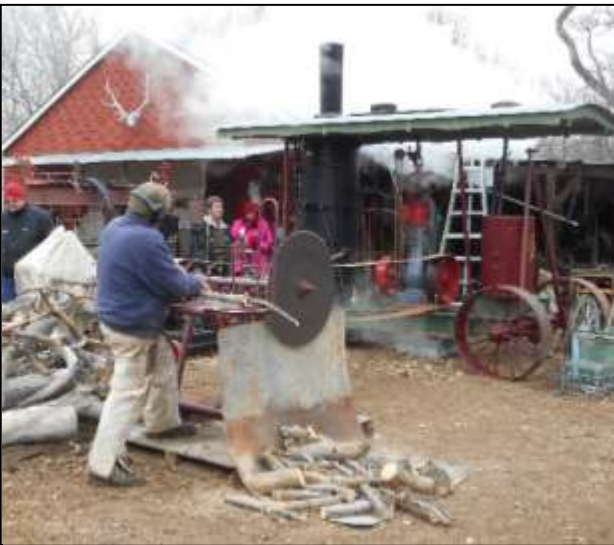
Above: Scott uses a circular saw driven by belt from steam engine in the background. Note the iron wheels and canopy on his custom built steam engine.
