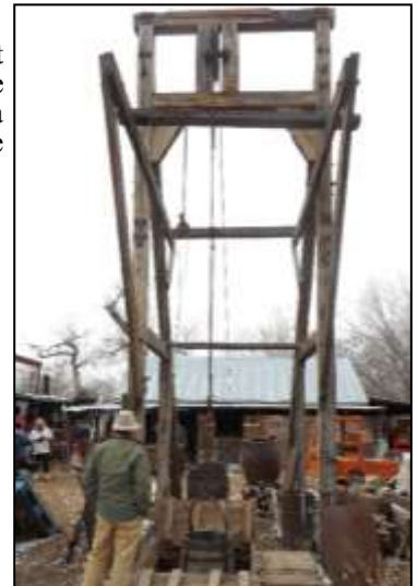
Above Right: A view of the hoist through the timber structure across the “mine shaft” to the shed housing the hoist engine and cable drum.
