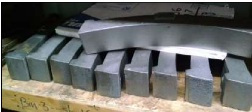
JUST ARRIVED: The new year brought delivery of new shoes for our baby. Above left are some of the shoes for the huge 80 inch drive wheels. The shoes at right are for the smaller wheels on the pilot truck and the rear truck under the cab and firebox.
