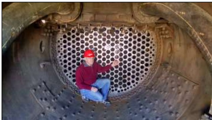
Insert Flue Tubes Here: Ernie Robart points to a clean, nicely polished front flue sheet.
