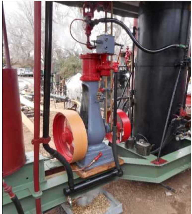
A Steamy Greeting For The New Year: Scotty Altenbach stands ready to start sounding a variety of steam whistles as Dan Toyama counts down to exactly noontime January 1, 2015. The whistles are mounted on a manifold connected to the boiler by a high pressure hose. Drive belt for saw is in foreground.
