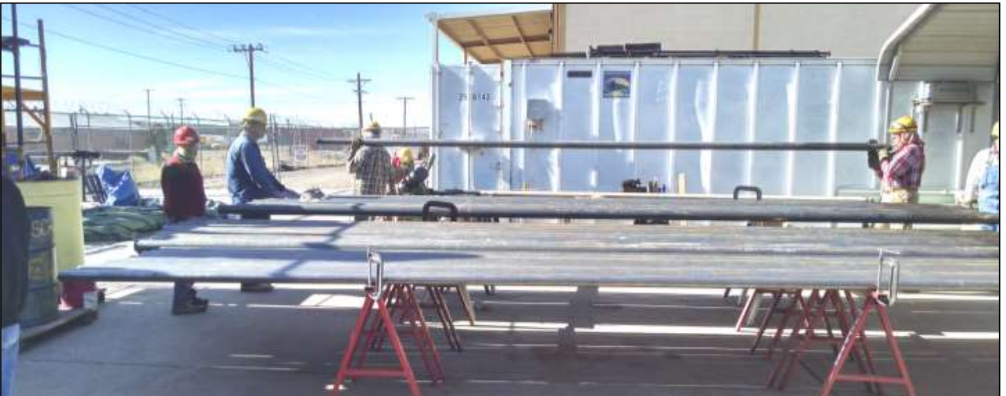
TOP: Flue tubes are removed from the storage container in background and racked for cleaning, inspection, and cutting to proper length.. BOTTOM: A metal wagon once used to haul parts about the Albuquerque Back Shops, is pressed into service as a work table where tubes can be securely clamped for accurate measurement and cutting with a metal saw. The fresh cut ends are cleared of metal burrs and the tubes are placed aside on racks to await insertion into the boiler.
