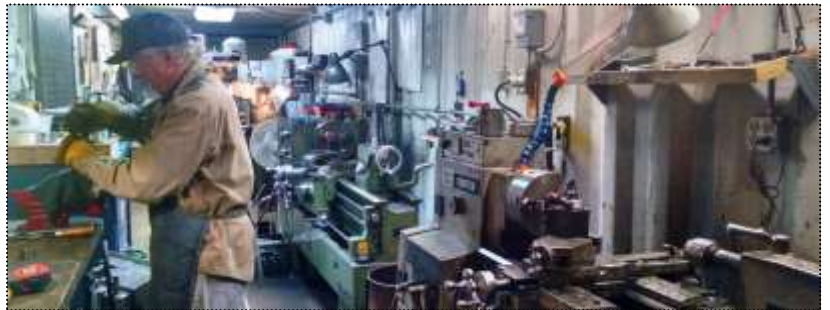
Above: With two lathes, a vertical mill, and numerous other donated machine tools, the 2926 machine shop is a bit cozy, but allows our machinists to accomplish a lot of work that would otherwise be shopped out at great expense. Here Ron Taylor is working at cleaning and checking bushings on brake linkage.
