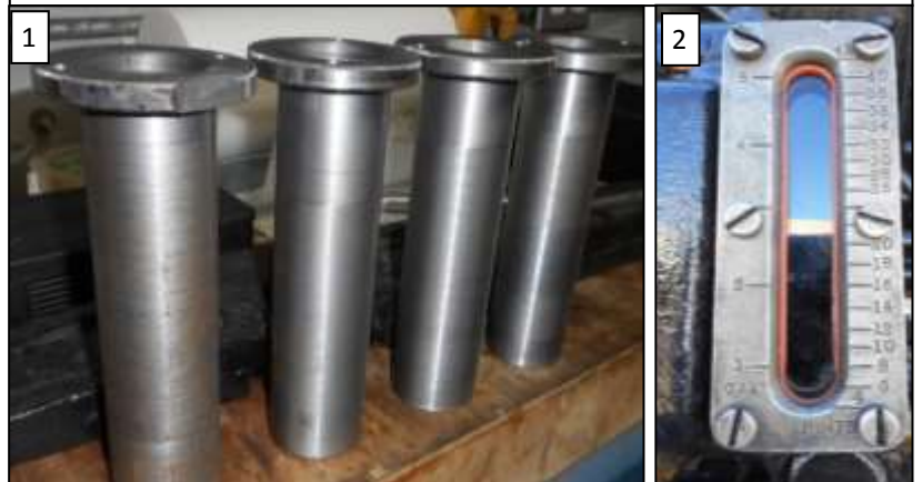
Below: Brake carrier pins, (1) produced in the machine shop and ready for use, and (2) The window is finally installed on the Nathan lubrication pump.
