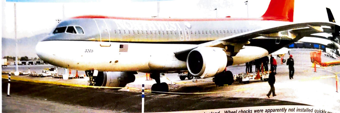
Apparently, this incident at Las Vegas/McCarran happened after the aircraft was towed to a remote stand. Wheel chocks were apparently not installed quickly enough, resulting in the aircraft rolling down the hill and sustaining damage to the rear underfuselage and wing trailing edge. (Patrick Dean)
