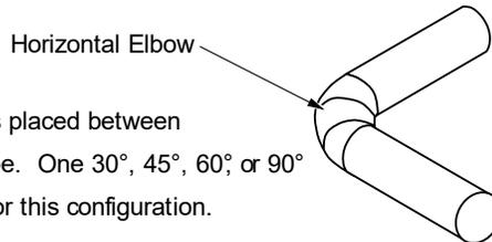
Horizontal elbows are elbows placed between two horizontal sections of pipe. One 30°, 45°, 60°, or 90° horizontal elbow is allowed for this configuration.
