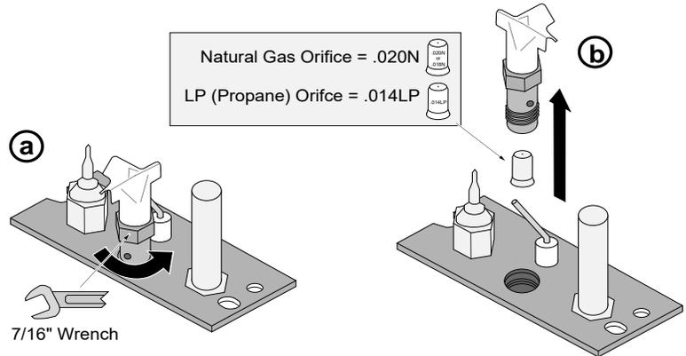
6. Remove the burner orifice and discard. Install the LP (propane) orifice.
