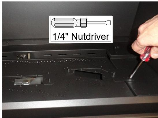
4. Remove the burner and place it aside.
