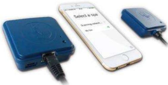
Each in.touch2 module has a status LED that can be used for troubleshooting purposes. The LED is located on the top of both enclosures.
