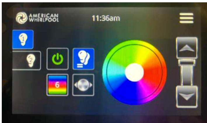
By default, in.mix selects Zone 1 when you access the menu. To lock both zones together, press the button with the two light bulbs. To unlock the two zones, press the same button again. Otherwise, adjust each zone by selecting the appropriate number on the left hand side.
