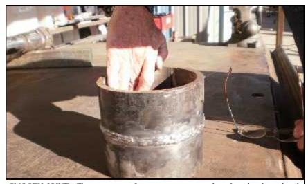
SMOOTH JOINT: The two pieces of pipe are now one, and ready to be cleaned, polished, and cut into strips called 'coupons'.
