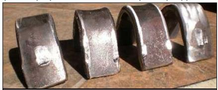
DANNY'S WINNING TICKET: These test strips, or 'coupons' are symbols of Danny Rivera's win over the difficult 6G test.
