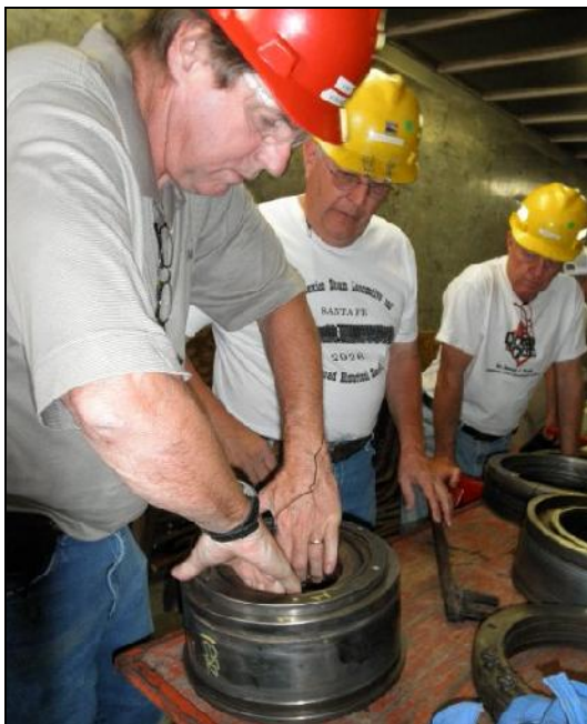
Dave Aungst, manufacturer's representative from Dallas checks a bearing as Bob DeGroft and Dave Van De Valde look on. Aungst was impressed with the condition of the bearings, after the locomotive's many years sitting in the park.
