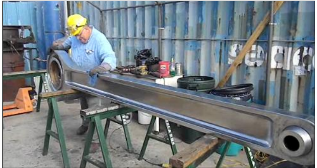
Above: Roger J. puts finishing touches on cleanup of a shiny 2926 side rod.
