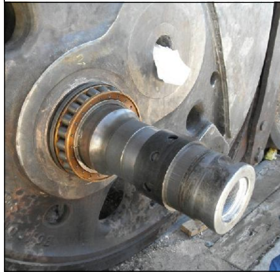
Below Left: One of many bearings still in place, awaiting puller. Right: Sanchez and Traudt work with one of the NMSLRHS custom built bearing pullers.
