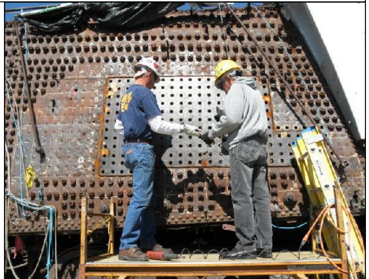
Above: Welding patches on the engineer's side wrapper sheet. Here, John G. and Danny R work (Left) inside and (Right) outside the firebox. Below: Next, on to the big patch on the fireman's side of the wrapper sheet.
