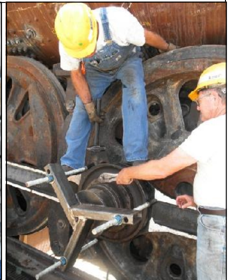
Below Left: One of many bearings still in place, awaiting puller. Right: Sanchez and Traudt work with one of the NMSLRHS custom built bearing pullers.
