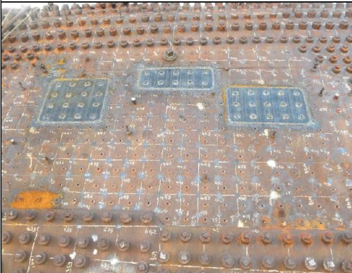
Above: Welding patches on the engineer's side wrapper sheet. Here, John G. and Danny R work (Left) inside and (Right) outside the firebox. Below: Next, on to the big patch on the fireman's side of the wrapper sheet.
