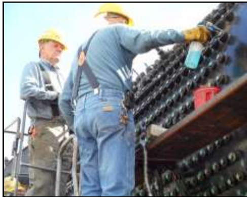
Finding and Fixing Those Pesky Leaks: 1. With 125 lb air pressure on the boiler system, Dave and Bob spray soapy water on neatly installed stay bolts. 2. Some leaks can be sealed with just a bit more torque on the bolt.
