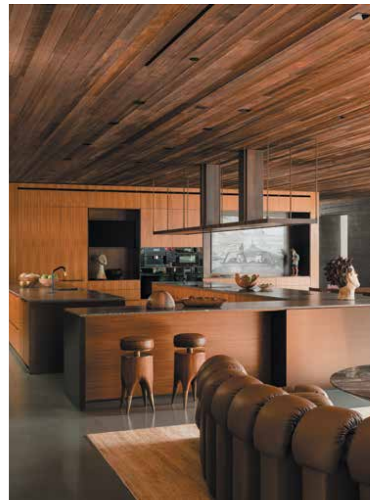
The kitchen's teak island is paired with stools from Blackman Cruz. A de Sede sofa sits atop a rug from Erik Lindstrom. Shou sugi ban, a Japanese process that consists of burning and then treating the wood, ensures the Douglas fir ceiling that runs throughout the home is mold-, bug-, and fire-resistant.
