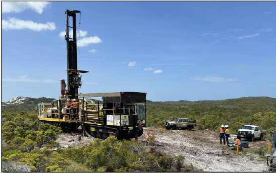
Figure 1: Sonic drilling rig completing groundwater bore drilling
