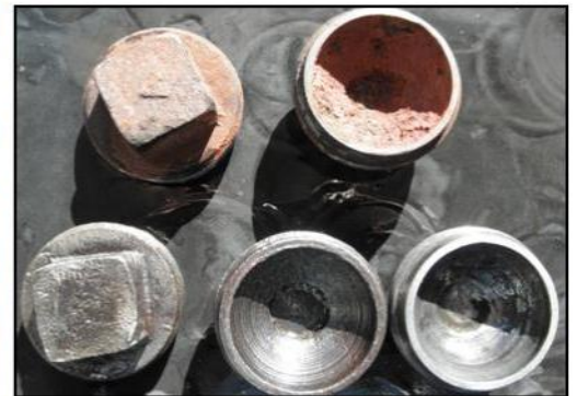
Before and after the cleaning process. The three lower caps are ready to reinstall.
