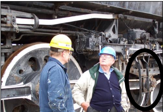
NMSLRHS Archive Photos: In the first photo, AT&SF retiree Glen Powers discusses the restoration with Dr. Mike Hartshorne before removal of the engineer's side crosshead. The area at far right (inside black oval) depicts the location of the crosshead assembly. Major components of the crosshead assembly are pinpointed in the second photo.
