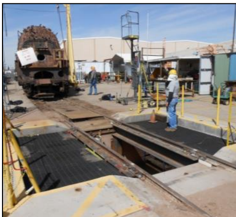
Left and Center: Lurch takes 2926 for a stroll, clearing the pit for a bit of cleanup before moving it back over the pit. Right: Once repositioned over the pit, flushing of the number three and four bearing reservoirs could be done,
