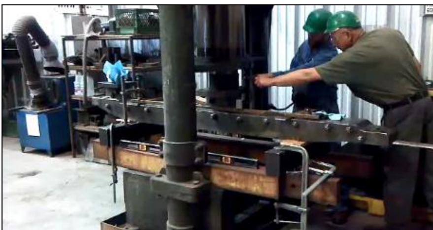
A view of the crosshead 'shoe' that contains the layer of Babbitt to provide a wear surface.
