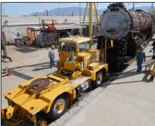
Left and Center: Lurch takes 2926 for a stroll, clearing the pit for a bit of cleanup before moving it back over the pit. Right: Once repositioned over the pit, flushing of the number three and four bearing reservoirs could be done,
