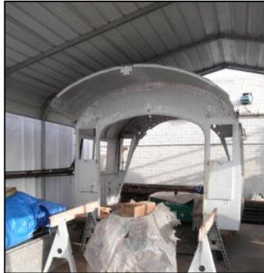
February 2012, Cab Move: The cab was lifted from 2926, placed under a canopy and measurements were made in preparation for installing the cab woodwork.
