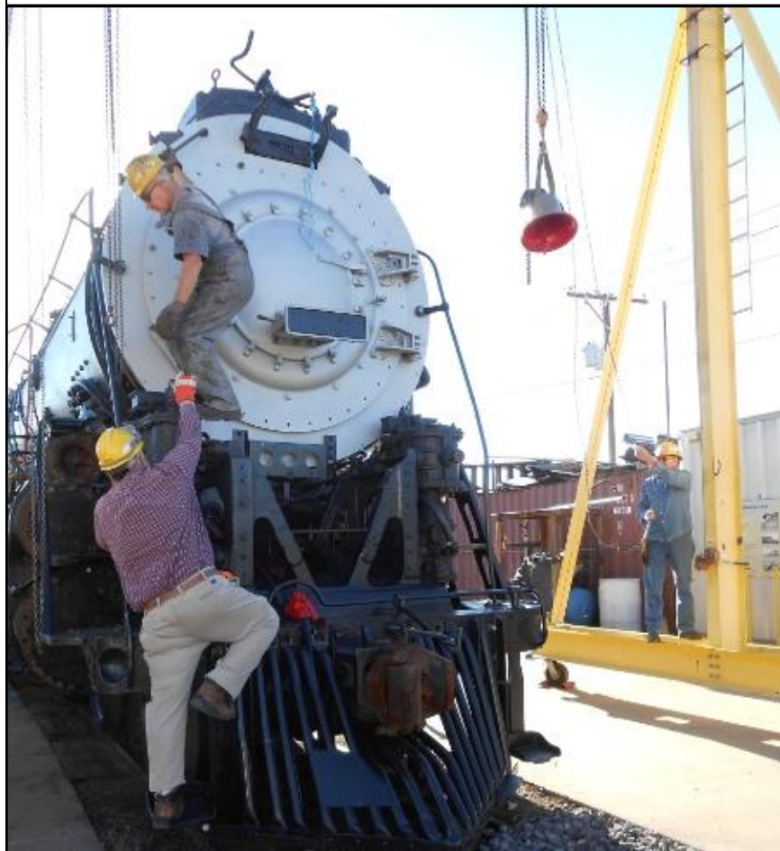
Below: Just about every part on 2926 is heavy, including the bell. Here, members are using gantry crane "Big Bird" to hoist and install the bell in its place at front of the locomotive, so the younger set could ring it. Once they ring the bell, they are presented by a certificate identifying them as members of the 2926 Ding-a-ling Club.
