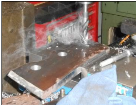
Using the pattern created from the 2912 cab bracket, raw material is cut and drilled to create pieces for welding.
