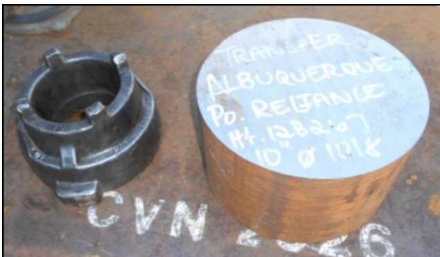
LEFT: A retainer borrowed from 2912 is pictured next to the large cylinder of steel that will be turned into a 2926 spring retainer by Eric. RIGHT: Two brand new finished retainers, with one snugly fit into its space on the buffer assembly.
