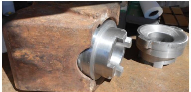
LEFT: A retainer borrowed from 2912 is pictured next to the large cylinder of steel that will be turned into a 2926 spring retainer by Eric. RIGHT: Two brand new finished retainers, with one snugly fit into its space on the buffer assembly.
