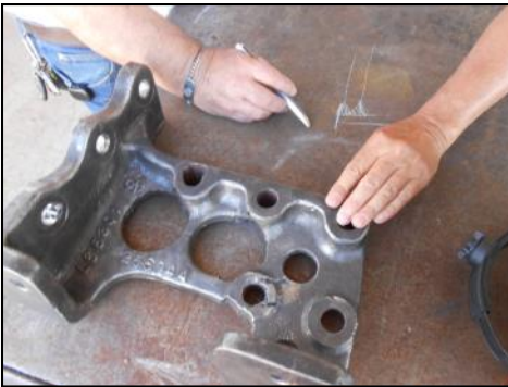
A cab bracket borrowed from the 2912 group in Pueblo is used to make a jig for fabricating one for 2926.
