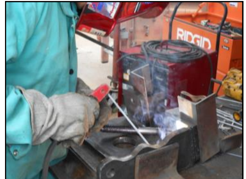
Jigged up on a welding table, the cut and drilled parts are welded into the final shape of the cab bracket.
