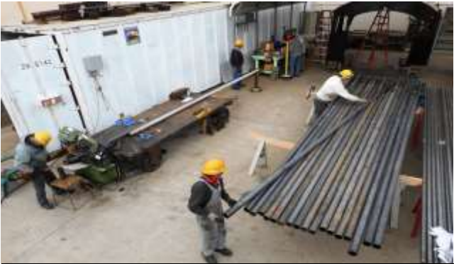
Above Left: With work underway on the 2926 cab under the canopy in the background, members of the flue tube crew prepare and rack flue tubes before beginning insertion into the boiler. Above Right: Lifting the tubes one at a time to team members on the scaffold next to the smokebox. Below Left: Scaffold team member Martin Sanchez steadies a flue tube on his shoulder while team inside smokebox inserts it into front flue sheet. Below Right: Task complete. Members of the scaffold team sign the last tube before passing it to the team in the smokebox.
