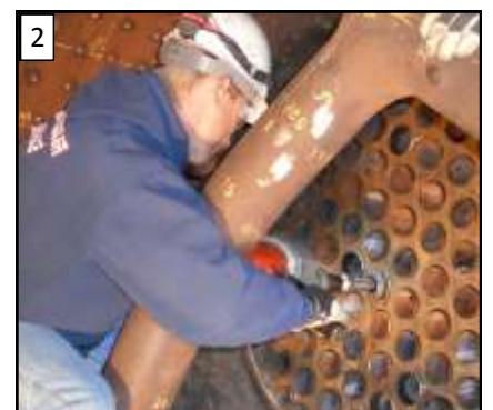
Welch boiler specialists at work: Photo 1, rolling tubes on the front flue sheet. The U-shaped devices at top are Superheater clamps. Photo 2, rolling tubes on the rear flue sheet. Ernie RobartPhotos:
