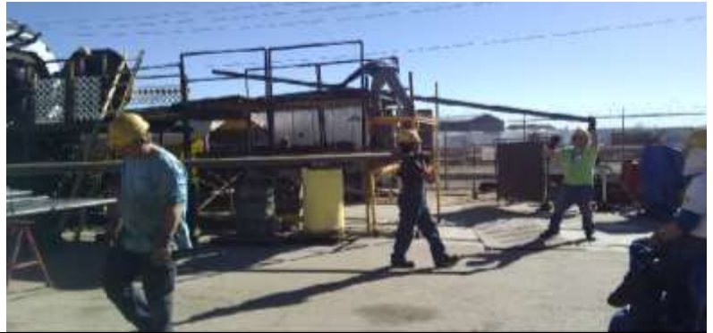
Above Left: With work underway on the 2926 cab under the canopy in the background, members of the flue tube crew prepare and rack flue tubes before beginning insertion into the boiler. Above Right: Lifting the tubes one at a time to team members on the scaffold next to the smokebox. Below Left: Scaffold team member Martin Sanchez steadies a flue tube on his shoulder while team inside smokebox inserts it into front flue sheet. Below Right: Task complete. Members of the scaffold team sign the last tube before passing it to the team in the smokebox.
