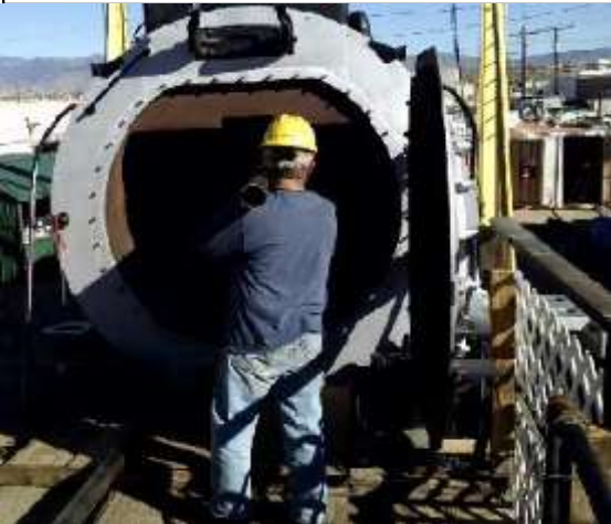
Above Left: With work underway on the 2926 cab under the canopy in the background, members of the flue tube crew prepare and rack flue tubes before beginning insertion into the boiler. Above Right: Lifting the tubes one at a time to team members on the scaffold next to the smokebox. Below Left: Scaffold team member Martin Sanchez steadies a flue tube on his shoulder while team inside smokebox inserts it into front flue sheet. Below Right: Task complete. Members of the scaffold team sign the last tube before passing it to the team in the smokebox.
