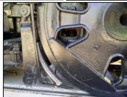
These pictures show just some of the brake parts. The table in the picture above holds an array of brake components. The parts will all be cleaned, tested, and assembled in the coming weeks. The brake stand at right is currently being modified to fit modern components. Below left: Some of the new cast iron brake shoes as they were unpacked on arrival. Below: Two views of new shoe installed on engineer side front drive wheel.
