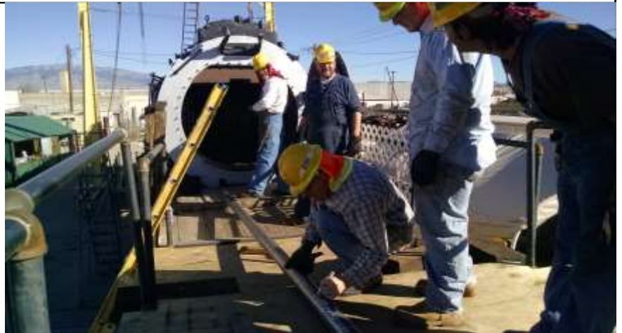
Above Left: With work underway on the 2926 cab under the canopy in the background, members of the flue tube crew prepare and rack flue tubes before beginning insertion into the boiler. Above Right: Lifting the tubes one at a time to team members on the scaffold next to the smokebox. Below Left: Scaffold team member Martin Sanchez steadies a flue tube on his shoulder while team inside smokebox inserts it into front flue sheet. Below Right: Task complete. Members of the scaffold team sign the last tube before passing it to the team in the smokebox.
