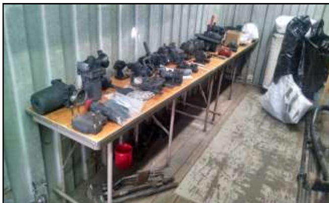
These pictures show just some of the brake parts. The table in the picture above holds an array of brake components. The parts will all be cleaned, tested, and assembled in the coming weeks. The brake stand at right is currently being modified to fit modern components. Below left: Some of the new cast iron brake shoes as they were unpacked on arrival. Below: Two views of new shoe installed on engineer side front drive wheel.
