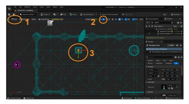
At this point, it's possible that your model may not be sitting precisely on top of the display. Switch to a left or right orthographic view to view your model's position on the display from the side. Use the Translate gizmo to adjust the position of the model up or down.
