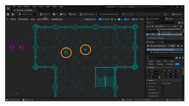
As in Perspective view, you can select an asset by clicking on it in the Viewport, or by clicking its name in the Outliner. Once selected, you can use the Translate and Rotate gizmos to move and rotate it. Note that your movement options are limited by the orthographic view you're using. In Top view, you can only move assets to the left and right, or from front to back. If you want to move an asset up or down, you need to use a front, back, left, or right orthographic view.
