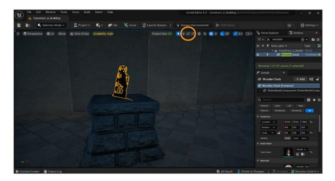
To make finer adjustments to the rotation, you may want to adjust the Rotation Grid Snap value, which defaults to 90 degrees. Locate the small angle measurement tool in the toolbar at the top right of the Viewport. Click on the angle icon to access a dropdown menu, and change the angle increment to a smaller number. This will allow you to rotate your model in smaller increments to achieve more precise positioning.
