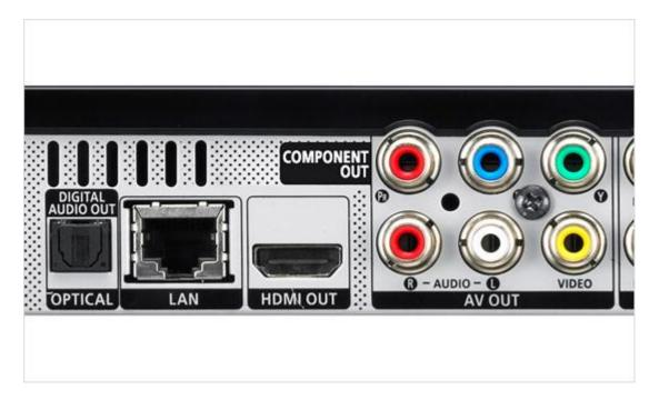
If you don't have an HDMI input on your HDTV, a component input is an older option which can still provide excellent HD quality from your player. Component video connections use three round cables with red, blue, and green ends next to each other. Any HDTV without HDMI has one or more component inputs. If you need to use a component connection with your TV, make sure that the Blu-ray player you buy has a component output (some newer Blu-ray players don't).
