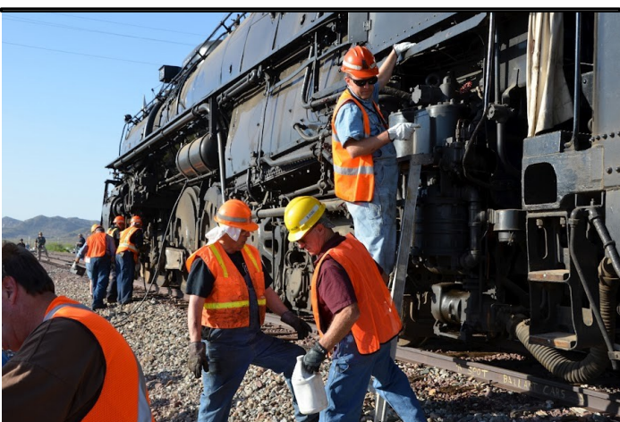
AT&SF 3751 crew member Ken Skolyan holds the ladder for Jim Campbell who is waiting for the jug of oil from NMSLRHS member Dave Van De Valde. The oil is for the rear cross-compound air compressor.
