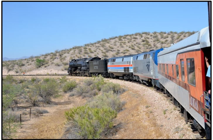
AT&SF 3751 and the two Amtrak P42 Diesels that provided extra traction when needed, and dynamic braking and head end power for the 14 cars of the consist.
