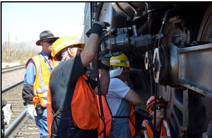
NMSL&RHS CMO Rick Kirby gets his time "shooting the rods," assisted by Gail Kirby reloading the grease. Amtrak's Eric Smith observes as his turn will be coming up. Matt Wiles watches below for tell-tale grease drip.
