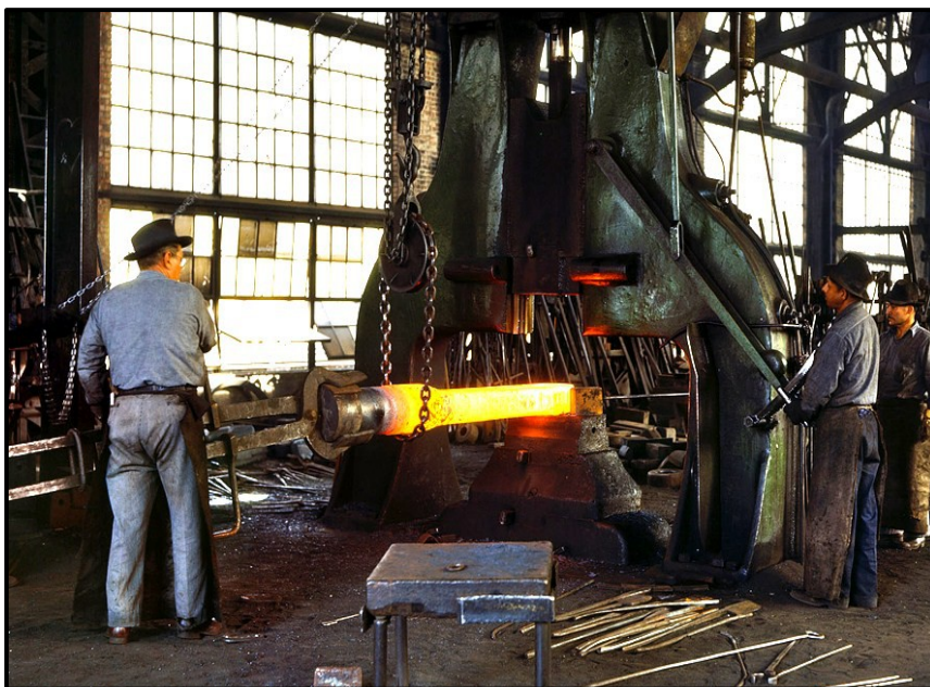
This is a rare photo of work inside the AT&SF Rail Shops in Albuquerque during WWII. Several shop employees are shown using the steam powered drop hammer to produce a steam locomotive drawbar from a round steel bar.
