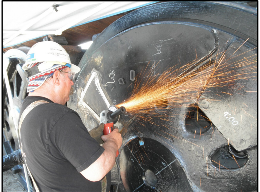
When 2926 was in operation during WWII and the Korean wars, time pressures and level of technology resulted in "less than optimum" welding when the locomotive was in the shop for repair. Now, with more time, better technology and the skills of a guy like Carlos, the old welds are ground away and replaced much finer work. Here Carlos grinds on old welds relating to counterbalancing the 80 inch drive wheels of 2926.
