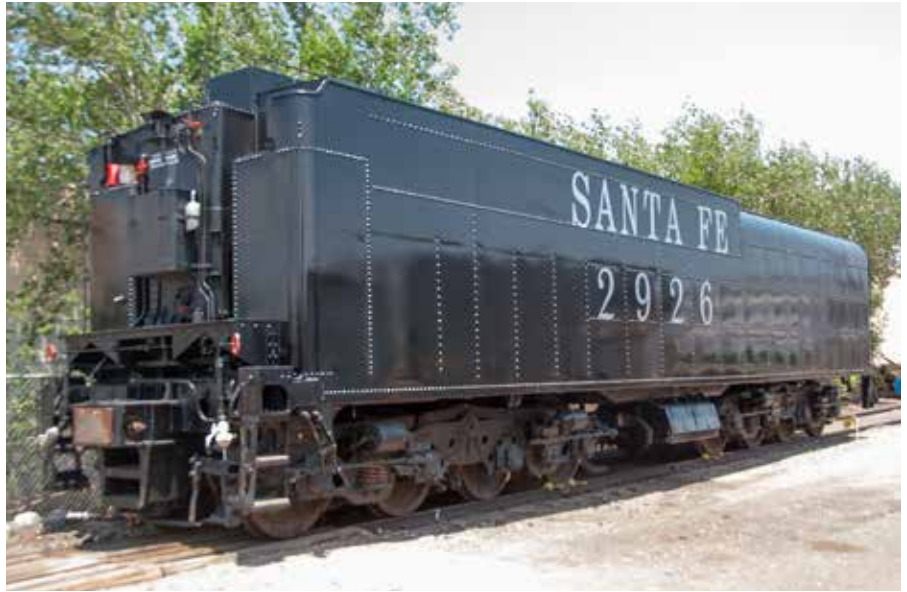
First major component to be completed was No. 2926's tender in 2011. The eight-axle rectangular tender holds 7,000 gallons of fuel oil and more than 24,000 gallons of water.
