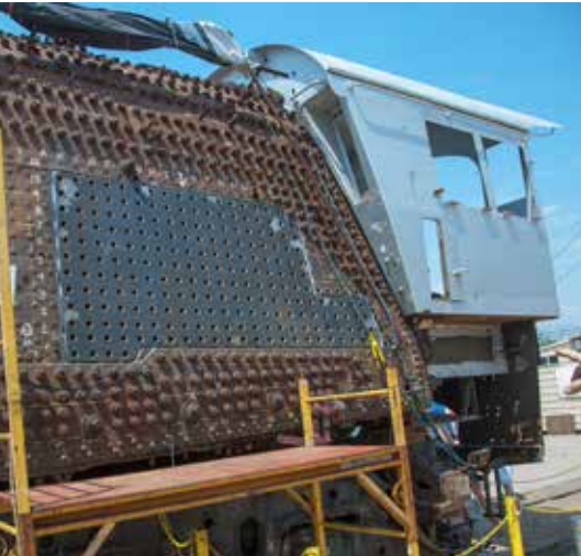
New boiler plate was installed on the fireman's side of the locomotive's firebox.
