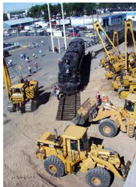
An ingenious “sand turntable” in a parking lot helped to get the locomotive out of Coronado Park. NMSL&RHS
