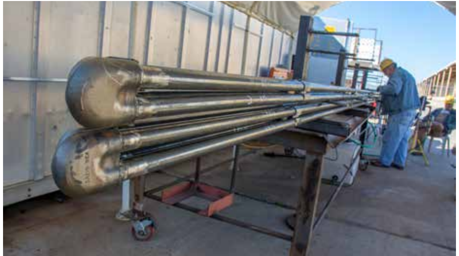
New superheater units are prepared for the boiler. The units were on display prior to installation at one of the New Mexico group's annual fall open houses. William P. Diven
