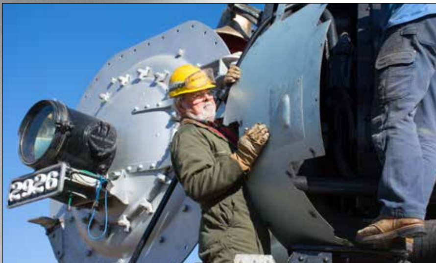
Running wide open and bound for Los Angeles, No. 2926 smokes up the skies near Victorville, Calif., in 1947, left. Above, volunteers with the New Mexico Steam Locomotive & Railroad Historical Society fit sheet-metal jacketing for the smokebox as the big 4-8-4 gets ready for the main line. Left, Western Railway Museum; above, William P. Diven
