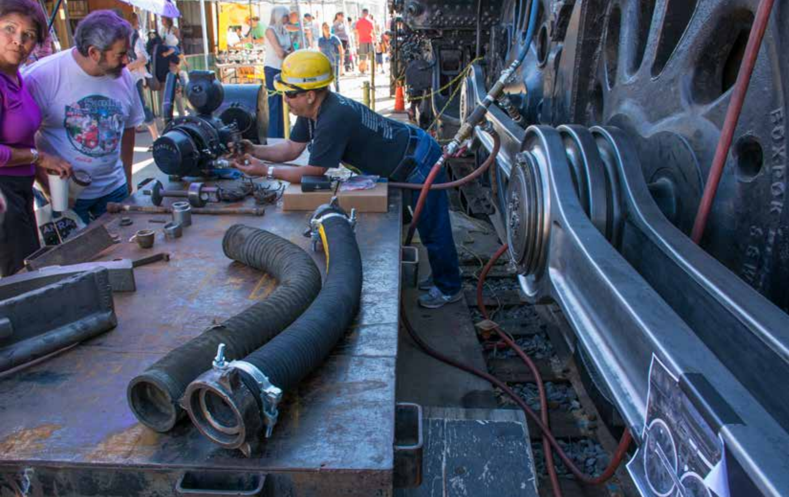
During an open house, volunteers on No. 2926 display and describe engine components within feet of the locomotive. On this table are tender hose connections, brake shoes, staybolt caps, turbo generator, and headlight, among many smaller parts. William P. Diven
