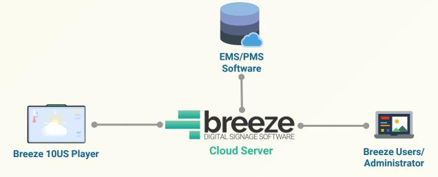
All communication in the Breeze architecture - whether it is the Feed Server to the Breeze Server Instance or Breeze Server Instance to individual players - occurs over HTTPS. HTTPS is HTTP connection secured with SSL/TLS.
