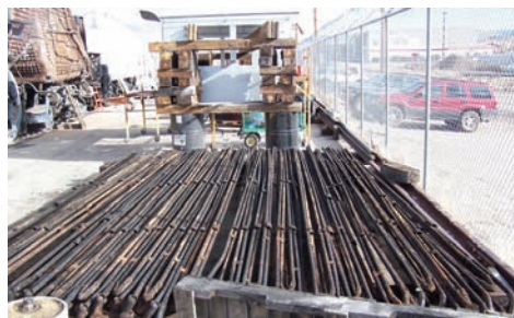
Stored Pipe Bundles: There are a lot of superheater pipes in a 2900 locomotive.
