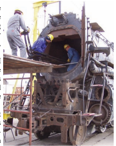
A bit of tugging, and a bundle of tubes emerges from the smokebox.
