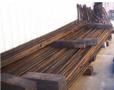
Stored Pipe Bundles: There are a lot of superheater pipes in a 2900 locomotive.
