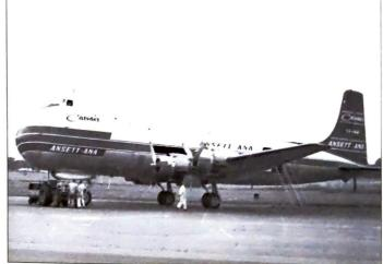
knots, however the rate of climb was slightly increased over the DC-4. This is attributed to the large nose, which produces some lift.
