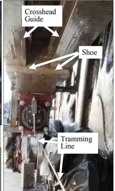
Figure 8, Above: Engineer side cylinder, front view., with center plate of hone in place.
