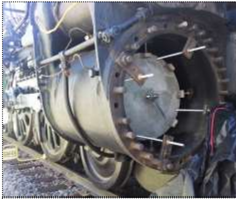
Figure 8, Above: Engineer side cylinder, front view., with center plate of hone in place.
