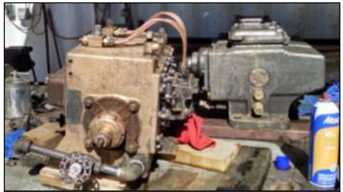
Figure 19: Two of the 2926 self lubrication units on workbench awaiting cleanup before reinstallation.
