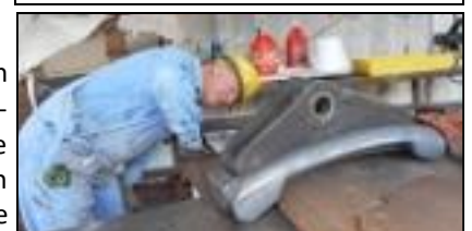
Above: The size of brake units is revealed by this brake shoe carrier. Below: New brake shoe mounted and properly adjusted can quickly turn these peanuts into peanut butter.
