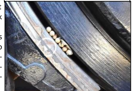
Above: The size of brake units is revealed by this brake shoe carrier. Below: New brake shoe mounted and properly adjusted can quickly turn these peanuts into peanut butter.
