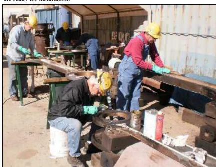
Busy Bees At A Side Rod Cleaning Party. The massive side rods, like all other parts are cleaned, polished and stored to await reinstallation. Meanwhile, their bearings are being thoroughly cleaned, and with guidance from Timken, will undergo a detailed inspection.
