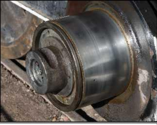
ABOVE: Removal of side rod reveals some nasty looking rust. Fortunately, it is not a bad as it looks, and cleans up well. BELOW: The hours of cleaning reveal beautiful shiny metal beneath the many layers of paint applied over 46 years of display on the park.
