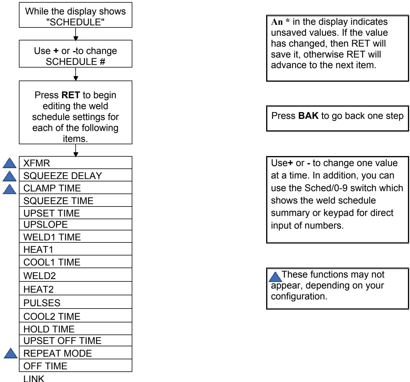
Once the Weld Controller has been configured for the specific application, it must be programmed with the welding functions available in the Edit menu. To program a **SCHEDULE** (a set of functions):
