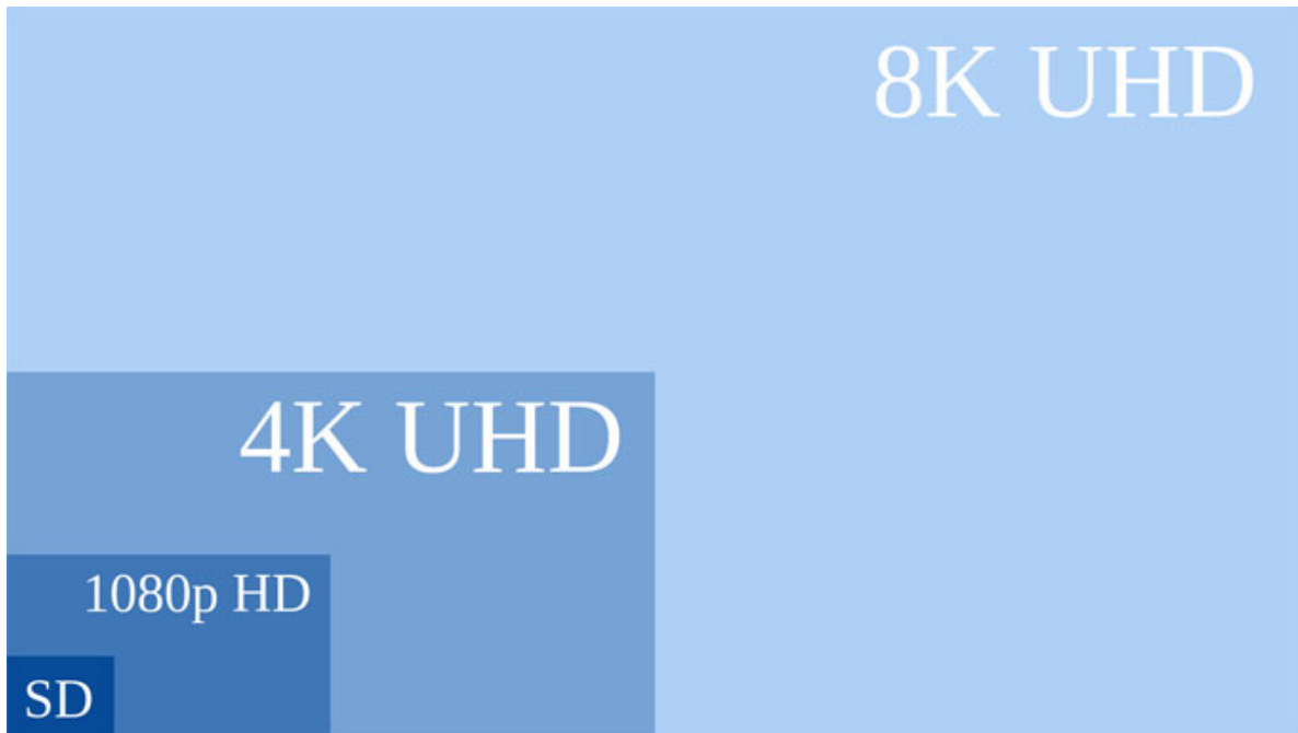
Ultra HD exists in two variants and both offers far more pixels than Full HD, picture from Wikipedia
