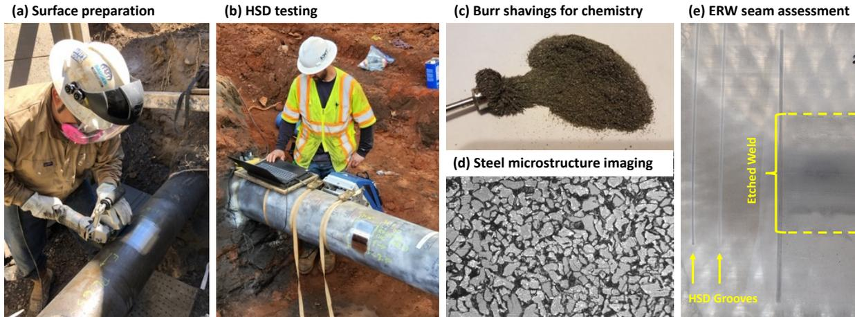
*Figure 6 Overview of in-ditch NDE methods. (a) Surface preparation is performed at suitable test locations. (b) The HSD is strapped to the pipe joint for testing. (c) Burr shavings are removed for chemical analysis. (d) The steel microstructure is etched and imaged. (e) Additional seam characterization is performed to assess the visual size of heat affected regions and mechanical variation in the weld.*
