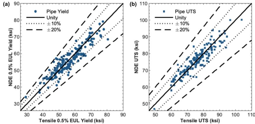
Figure 9 Unity plots comparing NDE and laboratory tensile measurements for (a) YS and (b) UTS
