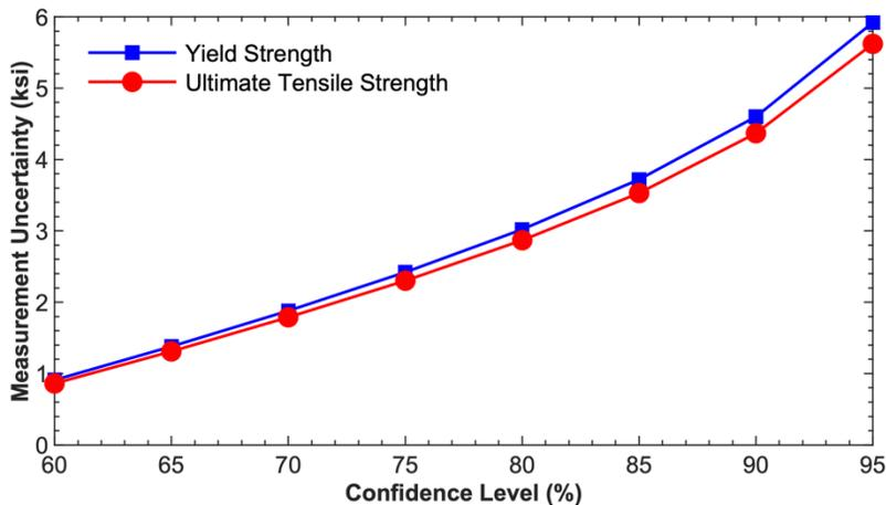
Figure 10 Strength measurement uncertainty of the HSD for varying confidence levels.
