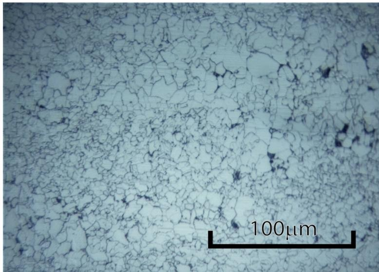
Figure 13 Pipe body microstructure image from in-situ metallography.
