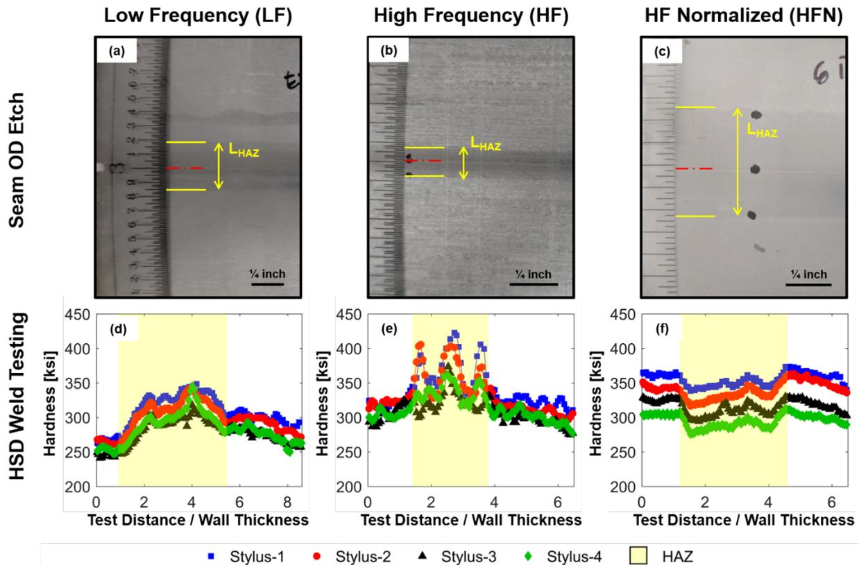
Figure 7 Representative etched seams (a-c) and hardness profiles (d-f) for LF, HF, and ~~HFN~~ HFN-ERW welds.
