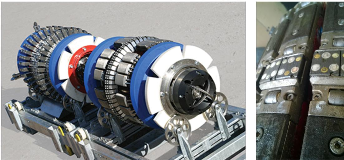
Figure 2 RoMat PGS Sensors and a standard MFL A ILI tool
