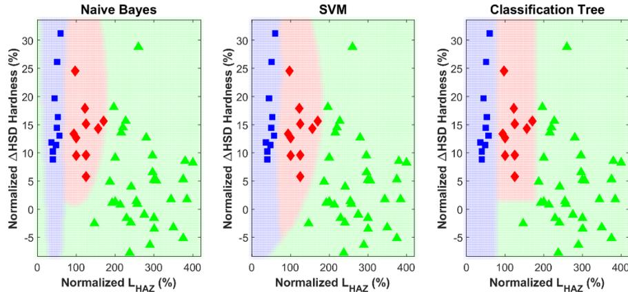
Figure 8 Seam classification for database of 54 unique ERW pipe samples. Blue indicates HF, red indicates LF, and green indicates HFN. Each plot is a different classification algorithm applied to the database, resulting in differences for the decision boundaries dividing the welding processes.
