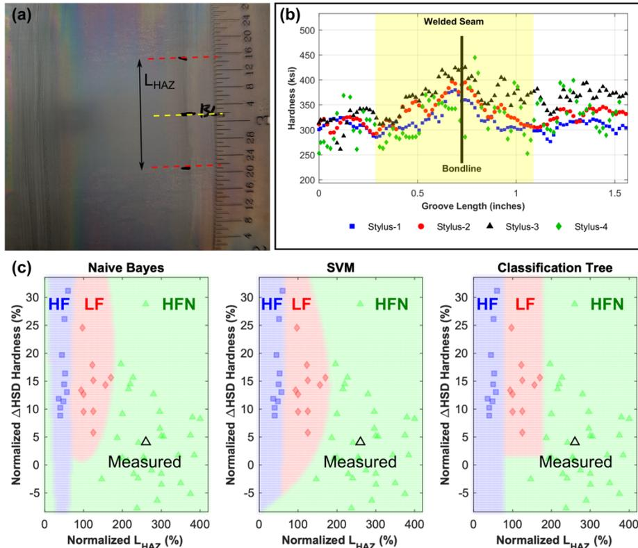
Figure 12 Overview of welded seam analysis including the (a) etched weld and (b) HSD weld test with the HAZ identified by the shaded region. (c) The measured results can be compared to the ERW database to see that all classification models determine the pipe joint to be HFN-ERW.
