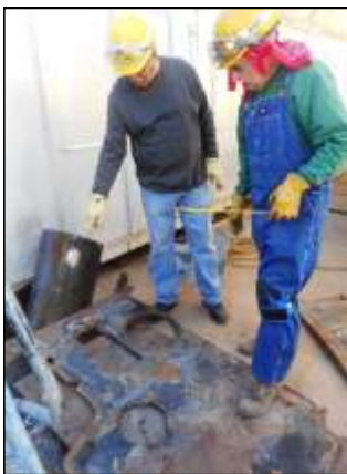
Right & Above: Sheet metal jacketing parts pulled from storage. The numbering helped, but the pattern making crew was still faced with a challenge.
