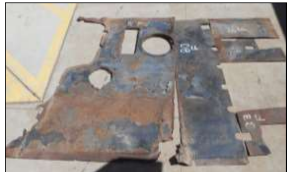
Above: Once the location of some of the large flat pieces of jacketing was identified, sheets of cardboard were used to create a pattern.
