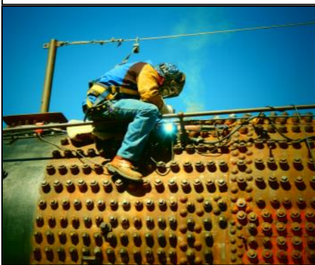
On top, on the side, or underneath, staybolt work was slow and tedious. It was also subject to a variety of weather conditions. Access, especially to those staybolts on the bottom would have been much simpler when 2926 was operating. In the bakshops, a large crane would have lifted the boiler from the locomotive frame, facilitating access to all staybolts without climbing or working in cramped spaces.
