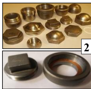
Repair and Replacement parts: (1) A selection of new staybolts. (2) New staybolt cap parts. Lower picture shows installation of copper gasket that was used in staybolt cap assembly. (3) Flexible staybolt assembly (4) Completed staybolts alongside original flexible and fixed staybolts.
