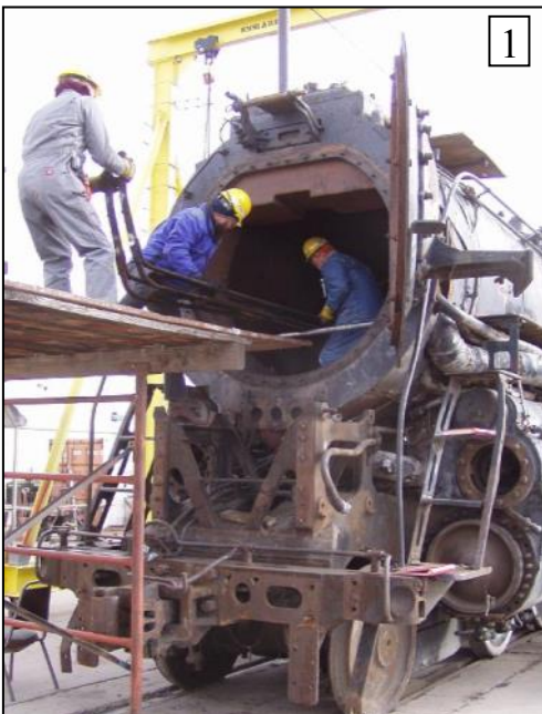
The double back feature (3) at the firebox end forms a pair. Two pairs are then connected before linking to the superheater header. That means four tubes (1) connected only at the smokebox end must be pulled at once. To clear the front flue sheet and smokebox they must be pulled directly forward their entire 20 foot length. A scaffold was positioned at the front of the locomotive, to allow a straight pull. The cumbersome, sooty assembly of four tubes required several pair of hands to be moved down from the scaffold.
