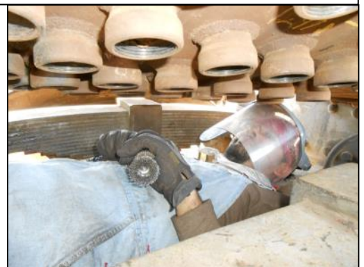
On top, on the side, or underneath, staybolt work was slow and tedious. It was also subject to a variety of weather conditions. Access, especially to those staybolts on the bottom would have been much simpler when 2926 was operating. In the bakshops, a large crane would have lifted the boiler from the locomotive frame, facilitating access to all staybolts without climbing or working in cramped spaces.
