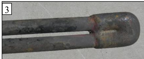
The double back feature (3) at the firebox end forms a pair. Two pairs are then connected before linking to the superheater header. That means four tubes (1) connected only at the smokebox end must be pulled at once. To clear the front flue sheet and smokebox they must be pulled directly forward their entire 20 foot length. A scaffold was positioned at the front of the locomotive, to allow a straight pull. The cumbersome, sooty assembly of four tubes required several pair of hands to be moved down from the scaffold.
