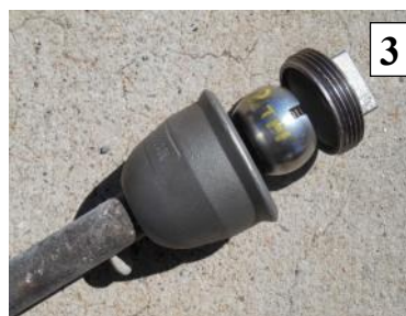
Repair and Replacement parts: (1) A selection of new staybolts. (2) New staybolt cap parts. Lower picture shows installation of copper gasket that was used in staybolt cap assembly. (3) Flexible staybolt assembly (4) Completed staybolts alongside original flexible and fixed staybolts.
