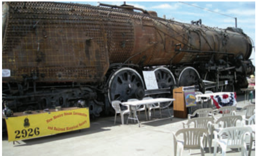
Bare Facts: AT&SF 2926, stripped of sheet metal cladding, asbestos insulation, accessories and appliances stands naked as it awaits distinguished visitors on April 8, 2008.
