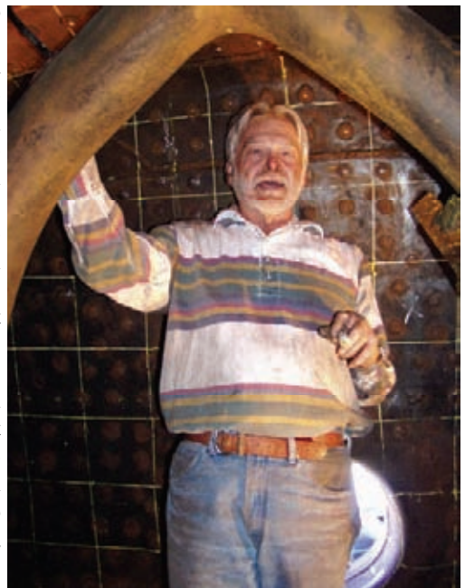
With marker in hand, Randy is caught inside 2926’s enormous firebox, where he is gridding the inside of the boiler’s wrapper sheet.
