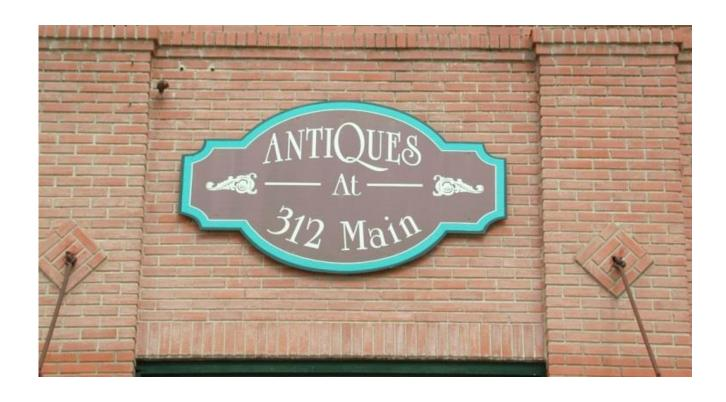
Note depth created by bracket mounting, contour cut and border outline
