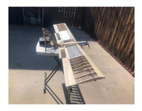
When not working at the 2926 or playing with grandkids, John is designing and constructing a solar-power drone. This remarkable plane has an almost 10-foot wingspan, a 14-inch foldable prop, and a 2.4 GHz computerized radio control system. All of this weighs in at just under five pounds, a remarkable achievement, at least from this author's point of view!
