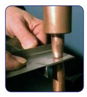
THE PROBLEM: Welding their parts required that the operators' fingers had to be close to the moving electrodes. Because of the part design and large number of different models being welded, there was no way they could use drop-in fixtures and antitiedown hand buttons.
