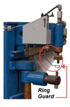
distance. At the start of each weld, the loop is sent downward before movement of the upper electrode. If the ring is stopped by a finger or other object before reaching the top of the part being welded, the limit switch does not trip and the electrode won't close.
