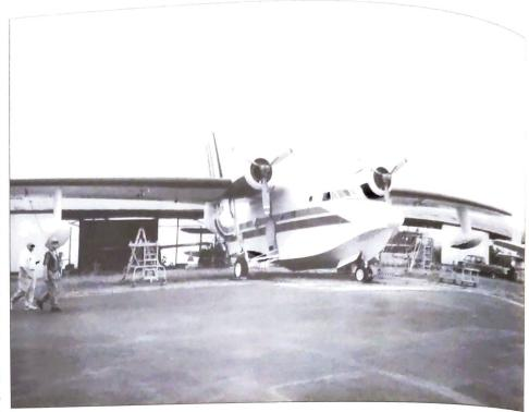
based in Miami. The extensive conversion included a zerotimed airframe, dual engine fire suppression systems, auto feather props, stainless steel oil tanks and titanium wing spar caps, and extra emergency exits. The G-111 was only in service a few years when Chalk's began withdrawing their fleet for economic reason, and parking them in the desert. Donald Trump gained financial control of the carrier, but the G-111s were not returned to service, opting instead for Grumman Turbo Mallards.
