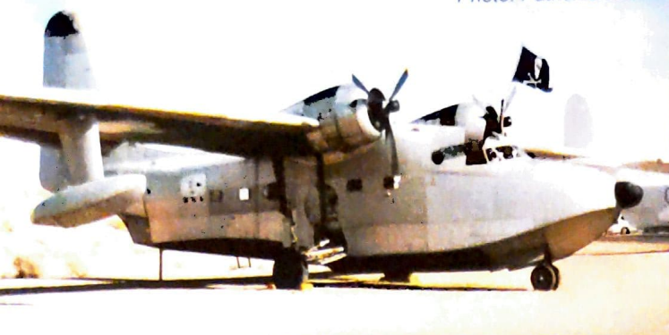
N117B is one of only 16 built with supercharged 1525 hp engines. Photo: Patrick Dean
