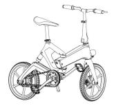
Folding the front wheel anticlockwise and folding the rear wheel clockwise
