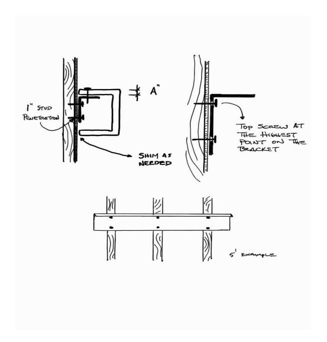
\*Picture below is if mantel is over metal on fireplace unit. Still finding 3 studs for 5ft and 4 studs for 6ft mantels.
